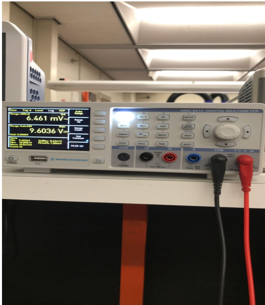
Figure 43: Voltage output of the solar panel while indoors through the multimeter
